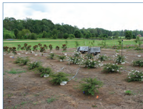
Automated Carbon Efflux System (ACES) installed adjacent to plants to continuously monitor C lost through soil respiration.
