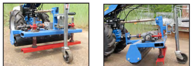
Figure 3. Powered roller/crimper for small, walk-behind two-wheeled tractors.
