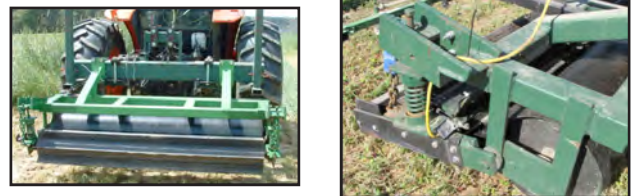
Figure 2. Two-stage roller/crimper. Smooth roller in front; Independent crimping drum in rear.
