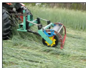
Figure 1. Rolling rye with the smooth roller (dark-color) with crimping bar (red).
