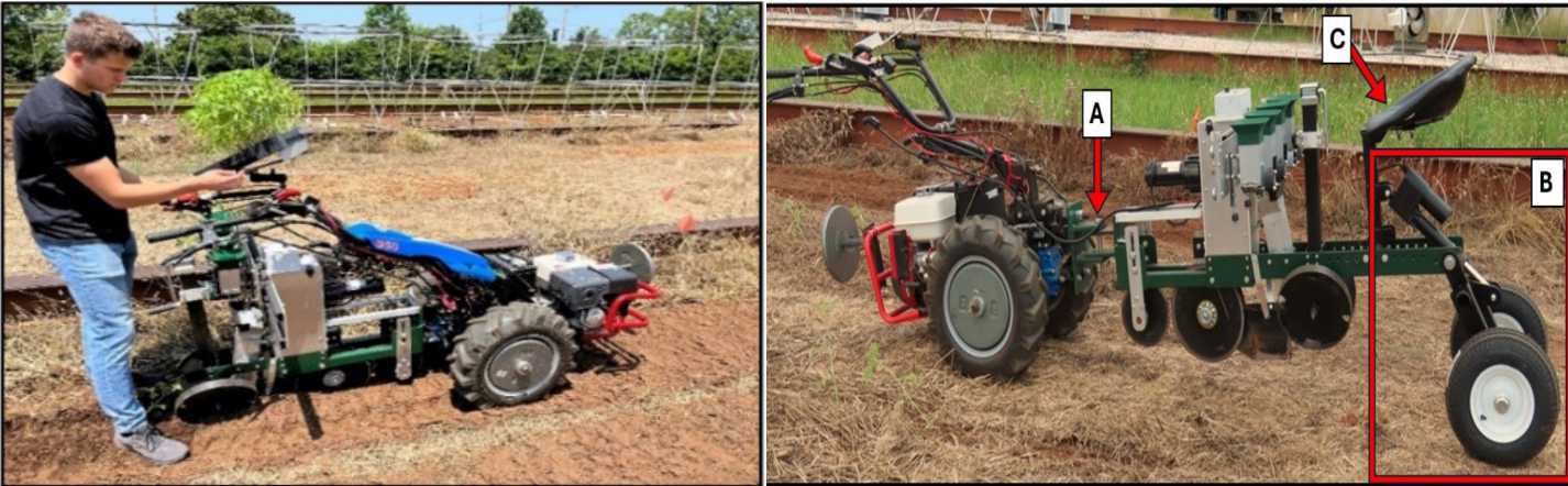
Fig. 3. Left: Version 1 (V1) seedling transplanter used in the first season. Right: Version 2 (V2) seedling transplanter used in the second season modified with (A) pivot point, (B) rear lift-assist wheels, (C) and seat for 2 nd operator.
