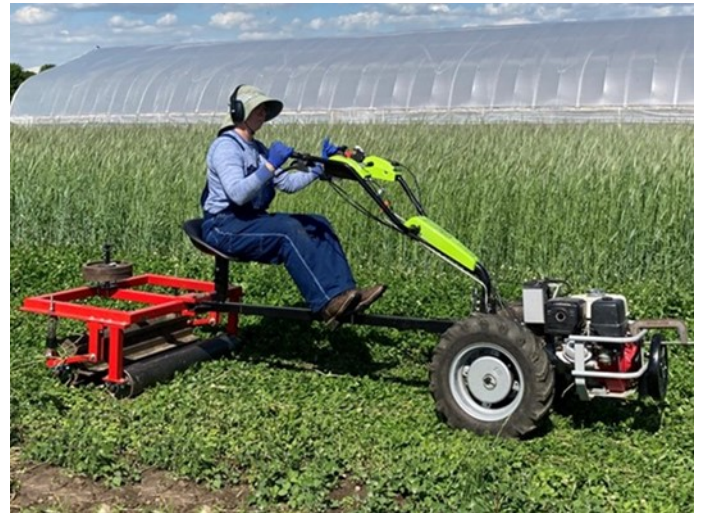
Figure 1. Two-stage roller/crimper (US patent #7,987,917 B1) for walk-behind tractors, ride-on version to improve operator's work effort and to increase effectiveness of crimping cover crop.
