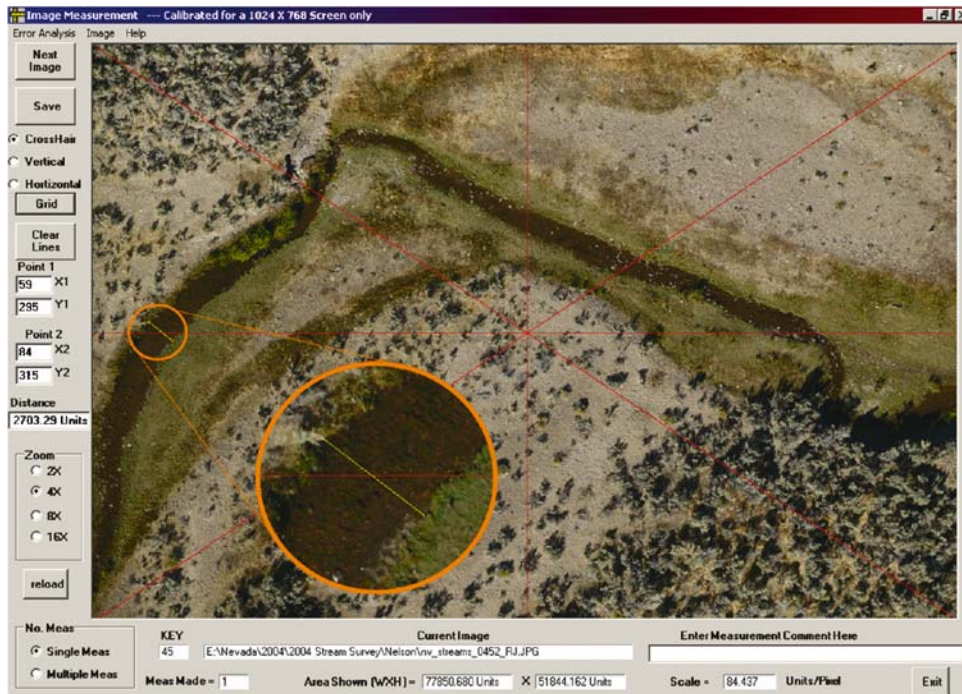
Figure 1. ImageMeasurement 1.0 screenshot showing a large scale aerial image of a stream in Wyoming. The image was acquired from 217.4 m above ground level using a Canon 1DS with 100 mm F/2.8 lens. Resolution for this image is 84.437 mm ground sample distance. Red crosshair-pattern gridlines are placed over the image and the point where the primary sample-location line intersects the center of the stream is used as the center of the yellow measurement line, which is placed perpendicular to stream flow. This stream has been measured at 2.703 m. The inlay shows the ability to zoom in for measurements, here shown at 4X. Other features of the software shown are the ability to apply vertical and horizontal line grids, the image footprint dimensions, the optional text comment box, different zoom level options and the toggle between single and multiple measurement modes.
