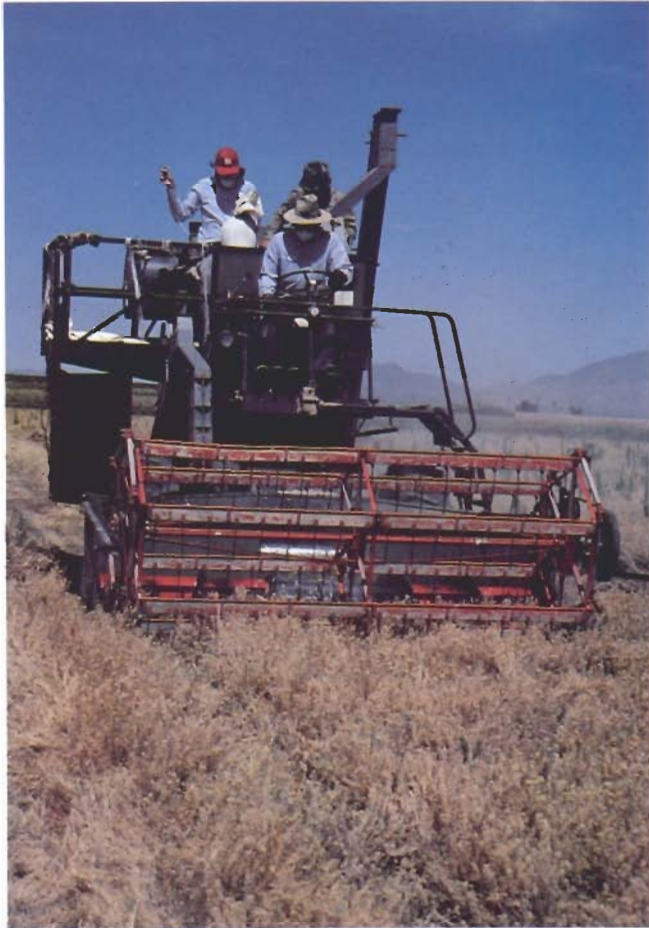
Lesquerella can be harvested with a small grain combine.
