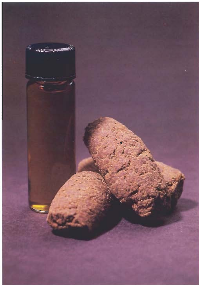
Extruded lesquerella collets prior to solvent extraction and a jar of oil.
