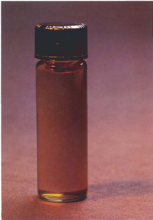
Lesquerella oil has a distinct reddish color; further bleaching studies are needed for some applications.
