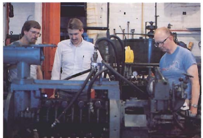
Pilot expeller processing lesquerella seed at the French Oil Mill Machinery Company, Piqua, Ohio.
