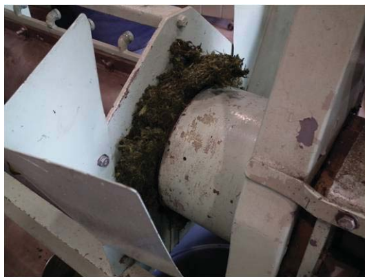
Press cake being made from leaf portion of alfalfa.
