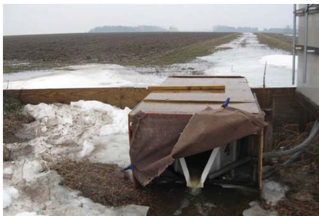
Research fields are designed so that runoff flows toward one of four flumes. The amount of flow is measured, and samples are collected.
