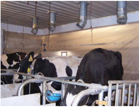
Air emission research is needed to measure and reduce the carbon footprint of milk production. Shown here is an air emission chamber at the USDFRC research farm.
