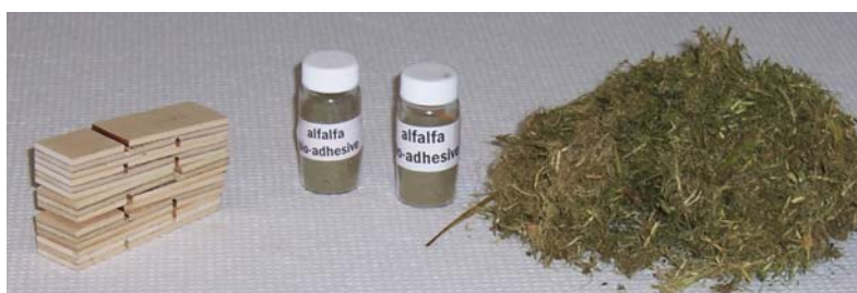
The USDFRC has discovered a residue product that could be used to produce a bio-based adhesive to replace phenol compounds in wood adhesives.
