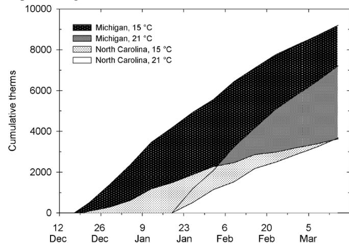
Figure 3. Relative amount of energy required to heat a 1,000 m<sup>2</sup> double-polyethylene greenhouse to produce nine bedding plant crops at four mean temperatures for two finish dates in MI, NY, and NC.
