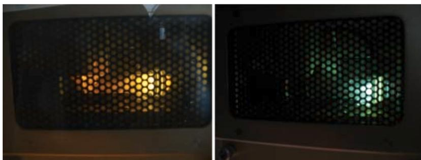
**Figure 4.** An ignited ICP-OES torch had an orange flame while analyzing samples with NaOH-digested plant tissue for Si analysis (A) but had a more typical green flame (B) when analyzing samples with KOH-digested plant tissue for Si analysis.
