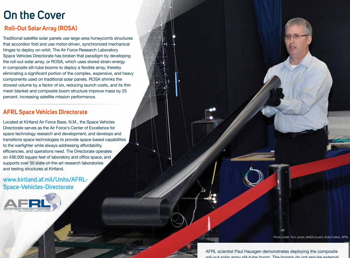
roll-out solar array slit-tube boom. The booms do not require external power, but deploy under their own stored-strain energy.
