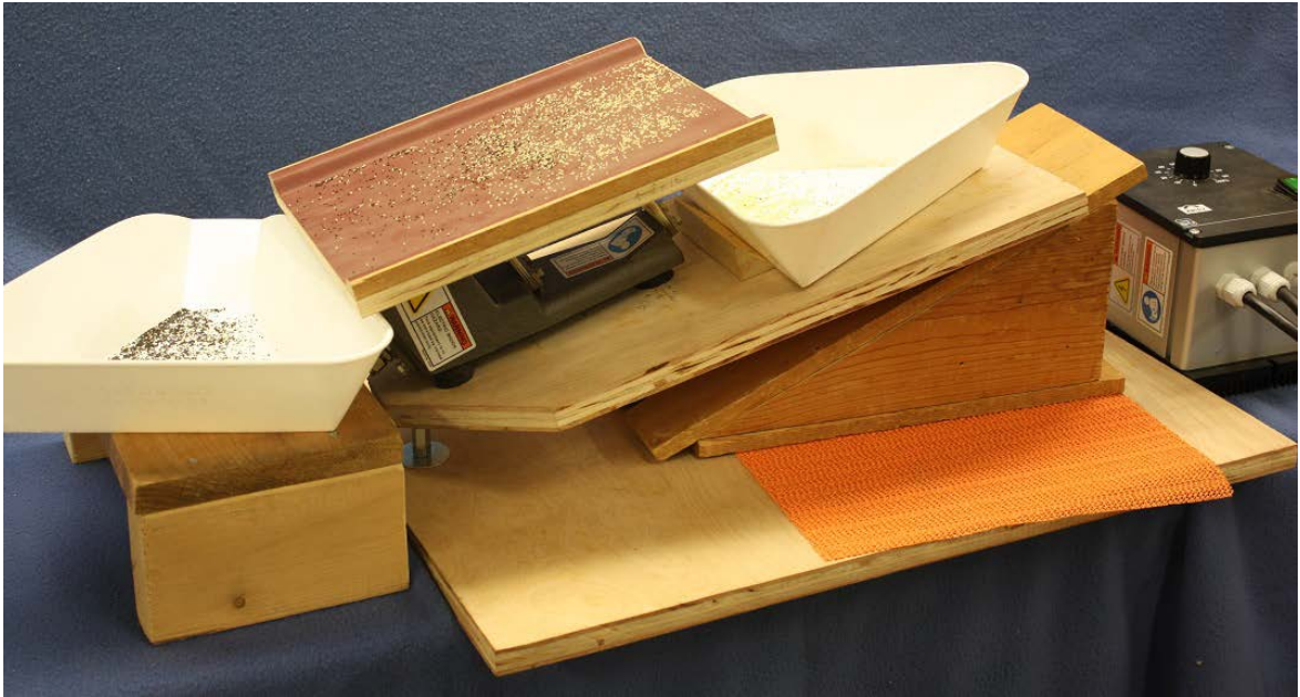
Figure 2. A vibratory deck seed cleaner with newly constructed wooden and plywood gear built by David Brenner and now in general multi-project seed cleaning use.
