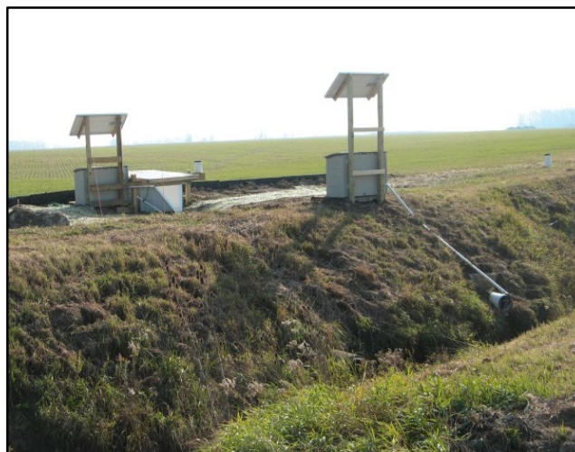
Edge-of-field site located in northwestern, OH, with surface runoff and subsurface tile drain monitoring
