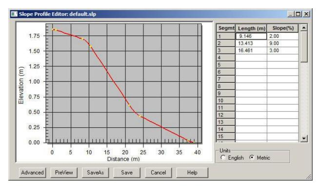
The yellow dots represent transition zones between slope segments. The default slope shape has 3 segments with slopes of 2%, 9% and 3%. Let's change the slope to a 100m uniform slope of 6%.
