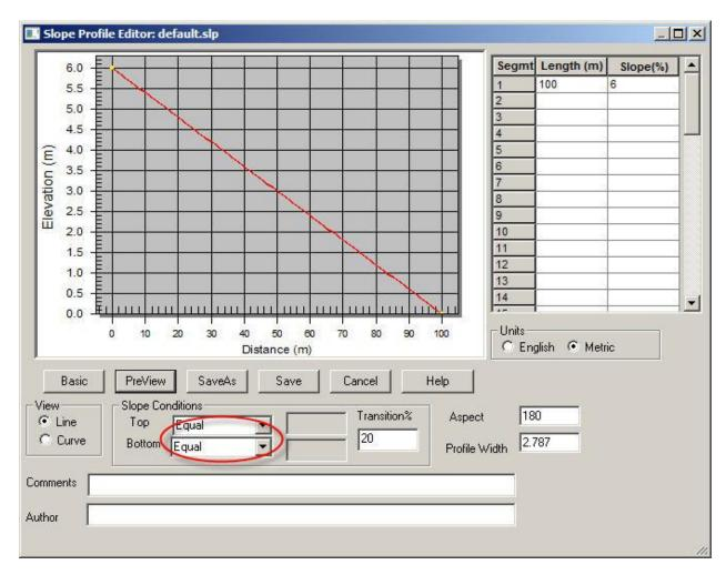
The aspect indicates the direction the slope is facing, in this case 180 is south facing. The parameter that can be set is the profile width. Change the profile width to 20m and the aspect to 90 and then click 'Save As' and name the file 'uniform-100-6.slp':
