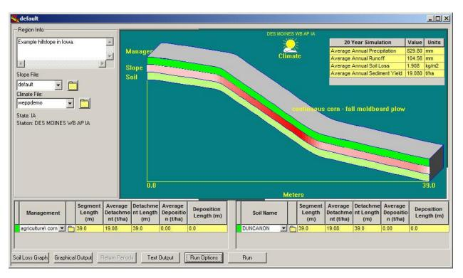
For the baseline condition the runoff was 104.56 mm/yr, soil loss 1.908 kg/m^2 and sediment yield 19.080 t/ha.
