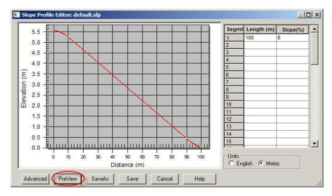
There are still two transition zones at the top and bottom. To make change these make the slope completely uniform click the 'Advanced' button to expand the window:
