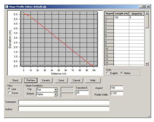
Next, change the slope conditions field to be 'Equal' which means it is equal to the adjacent slope segment. In this example 6%. Then click the 'Preview' button to display the updated slope profile.
