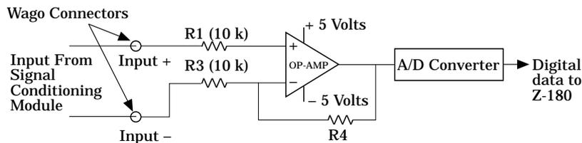
All of the above circuitry is contained on the Z-180 board itself for pressure measurement.
