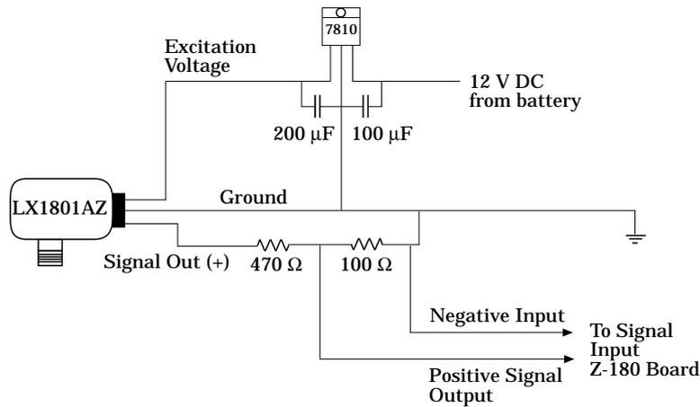
All of the above circuitry is located external to the Z-180 board for pressure signal conditioning.
