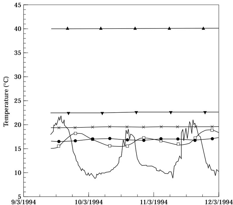
Fig. 3. Example plot of temperature system data on 9–12 March 1994 at Olinda Landfill, California, U.S.A. —, air temperature; ●, 50 cm; ▼, 152 cm; □, 7 cm; ×, 80 cm; ▲, 610 cm.
