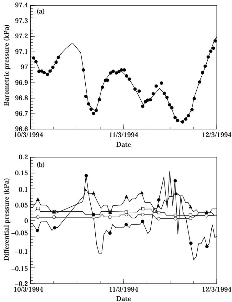
Fig. 5. Example plot of pressure system data using 163SC01D48 transducers on 10–12 March 1994 at Olinda Landfill, California, U.S.A. (a) —, barometric pressure. (b) ○, 25 cm; □, 100 cm; ▲, 310 cm; ●, 620 cm.
