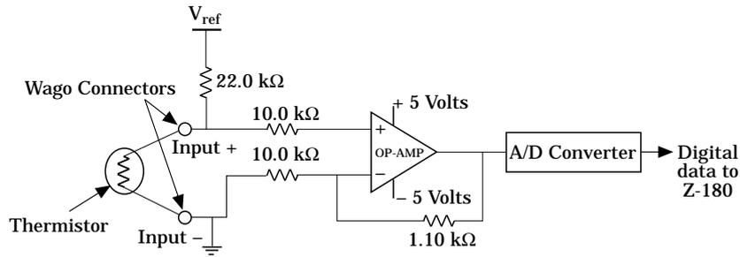
All of the above circuitry is located on the Z-180 board itself for temperature measurement.
