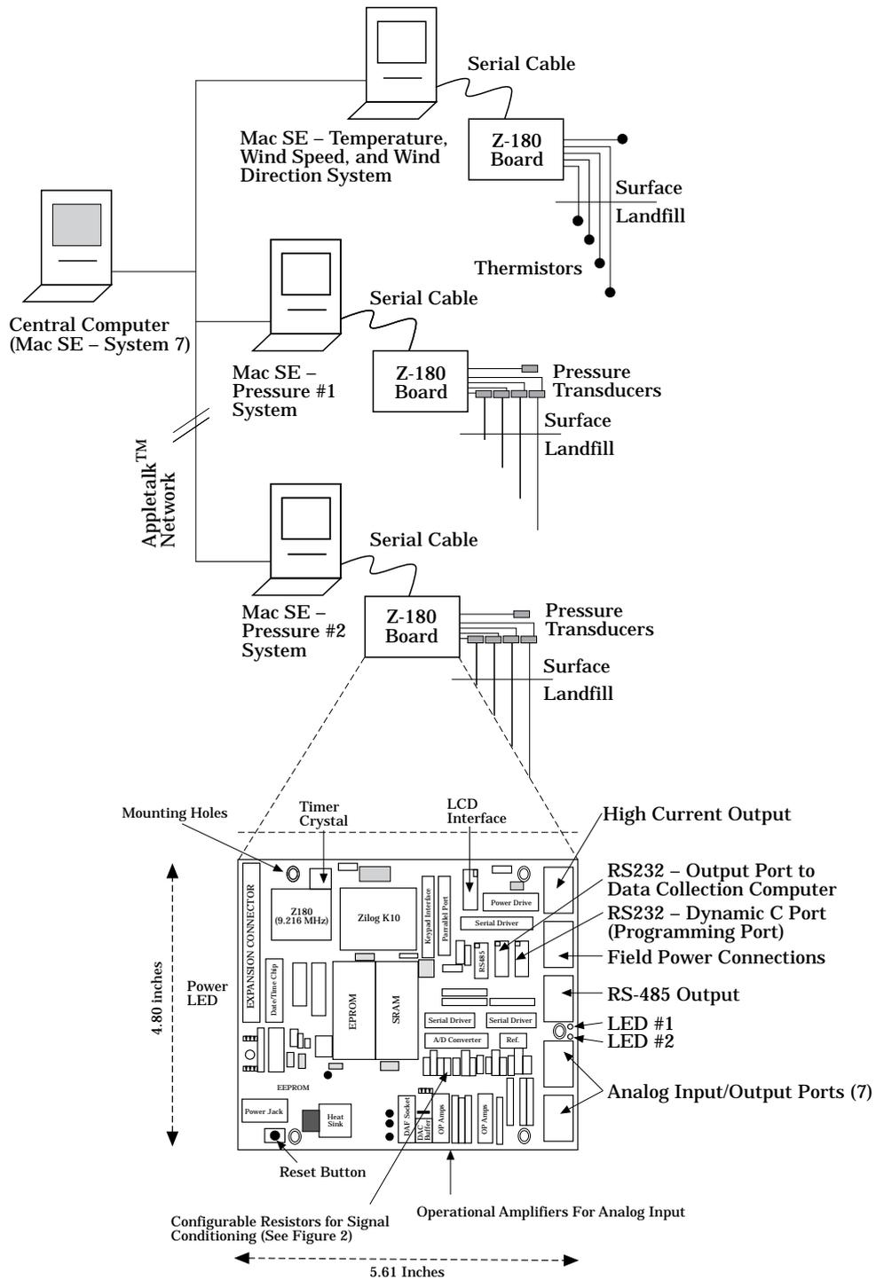
Fig. 1. Layout of data acquisition system and illustrations of features on Z-180 controller board.
