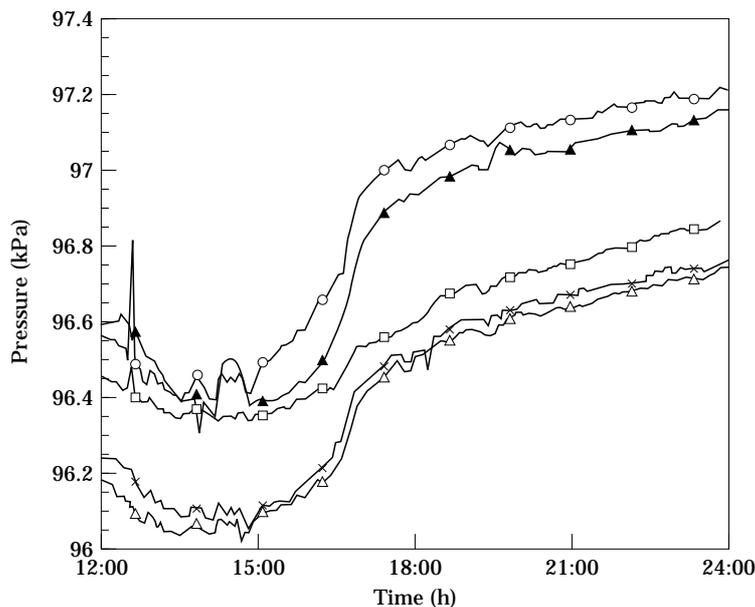
Fig. 4. Example plot of pressure system data using LX1801AZ transducers on 15 December 1993 at Olinda Landfill, California, U.S.A. ○, 25 cm; □, barometric pressure; ▲, 152 cm; ×, 610 cm; △, 40 cm.
