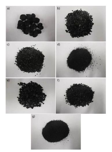
**Figure 1:** Photos of different particle sizes of Macadamia nutshell (a-d) and Pine chip (e-g) biochar used in this experiment: (a) 18mm, (b) 8.0-4.0mm, (c) 4.0-2.0mm, (d) <2.0mm, (e) 8.0-4.0mm, (f) 4.0-2.0mm, (g) <2.0mm.
