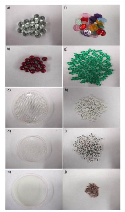
**Figure 2:** Photos of different particle sizes of spherical beads (a-e) and non-spherical beads (f-i): (a) glass 15.0mm, (b) plastic 8.0mm, (c) glass 3.0mm, (d) glass 1.0mm, (e) glass 0.1mm, (f) glass 13.0mm (13.0x18.0x2.0mm), (g) plastic 10.0mm (10.0x10.0x4.0mm), (h) plastic 7.0mm (7.0x7.0x2.0mm), (i) plastic 6.0mm (6.0x6.0x4.0mm), and (j) plastic 2.5mm (2.5x2.5x2.0mm).
