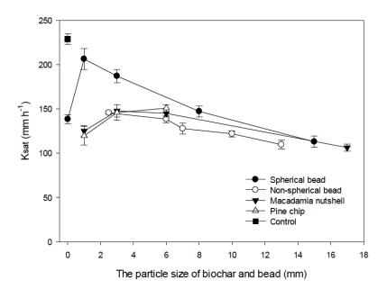
Figure 3: The comparison of saturated hydraulic conductivity between biochar (pine chip and macadamia nutshell) and beads (spherical and non-spherical bead) treated with different particle sizes on the medium sand.
