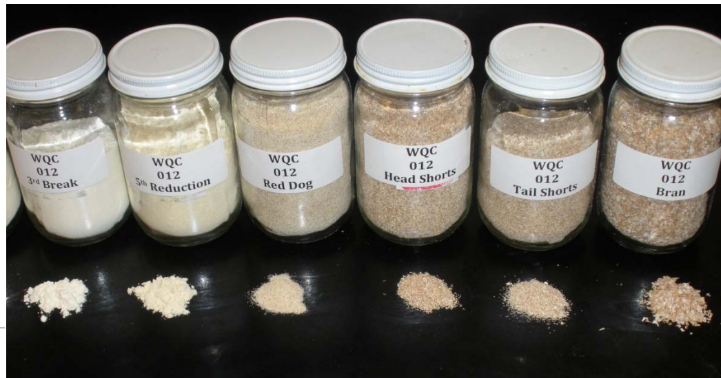
Reduction and bran streams from Miag mill
