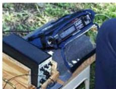
**Fig. 1B.** Example of test to monitor *C. formosanus* activity at an oak tree. S1-S4 indicate probes inserted into or near the tree. Accelerometer is shown at S3. Sounds detected easily at S3 were detected only faintly at S2 or S4 (15 cm away).
