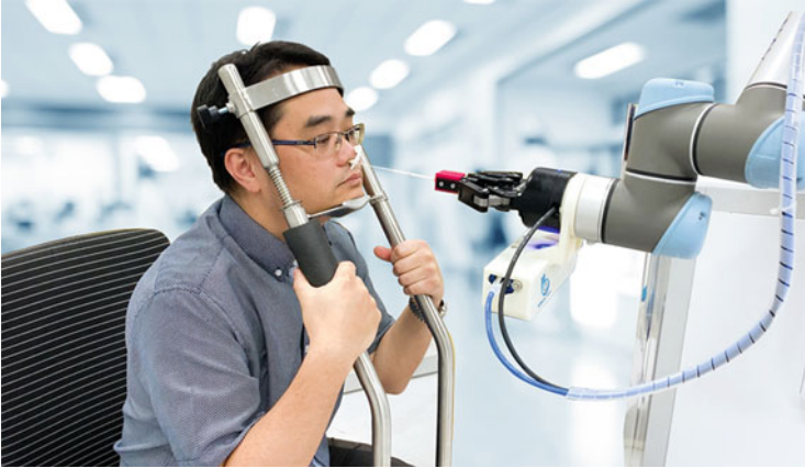
Fig. 20.10 Brain Navi, a Taiwanese firm, created a robot in just 8 weeks that collects a nasal swab sample, from a potentially infected COVID-19 patient, without putting the healthcare worker at risk, in just 2–5 min and then places the sample in a container for safe handling. (This photo was provided by Zoe Lee from Brain Navi with permission)
