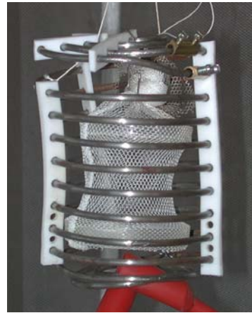
Fig. 2 - Helical metal zapper screen cages (dia. 50 mm by 80 mm)..
