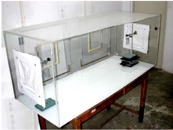
Fig. 1 - Plexiglas chamber equipped with speaker attachments (calling medfly males and control cage in both sides of the chamber).
