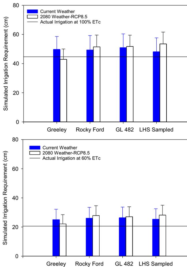
**Fig. 6.** Simulated actual evapotranspiration, AET, with current and proposed cultivars, averaged over 22 years. For LHS sampled cultivars, the results were averaged over 70 cultivars. Top: 100% ETC. Bottom: 60% ETC. Average simulated AET for the four year experimental data (2008–2011) at 100% and 60% ETC was plotted as reference. ETC: Crop Evapotranspiration. AET: Actual Evapotranspiration. LHS: Latin Hypercube Sampling.
