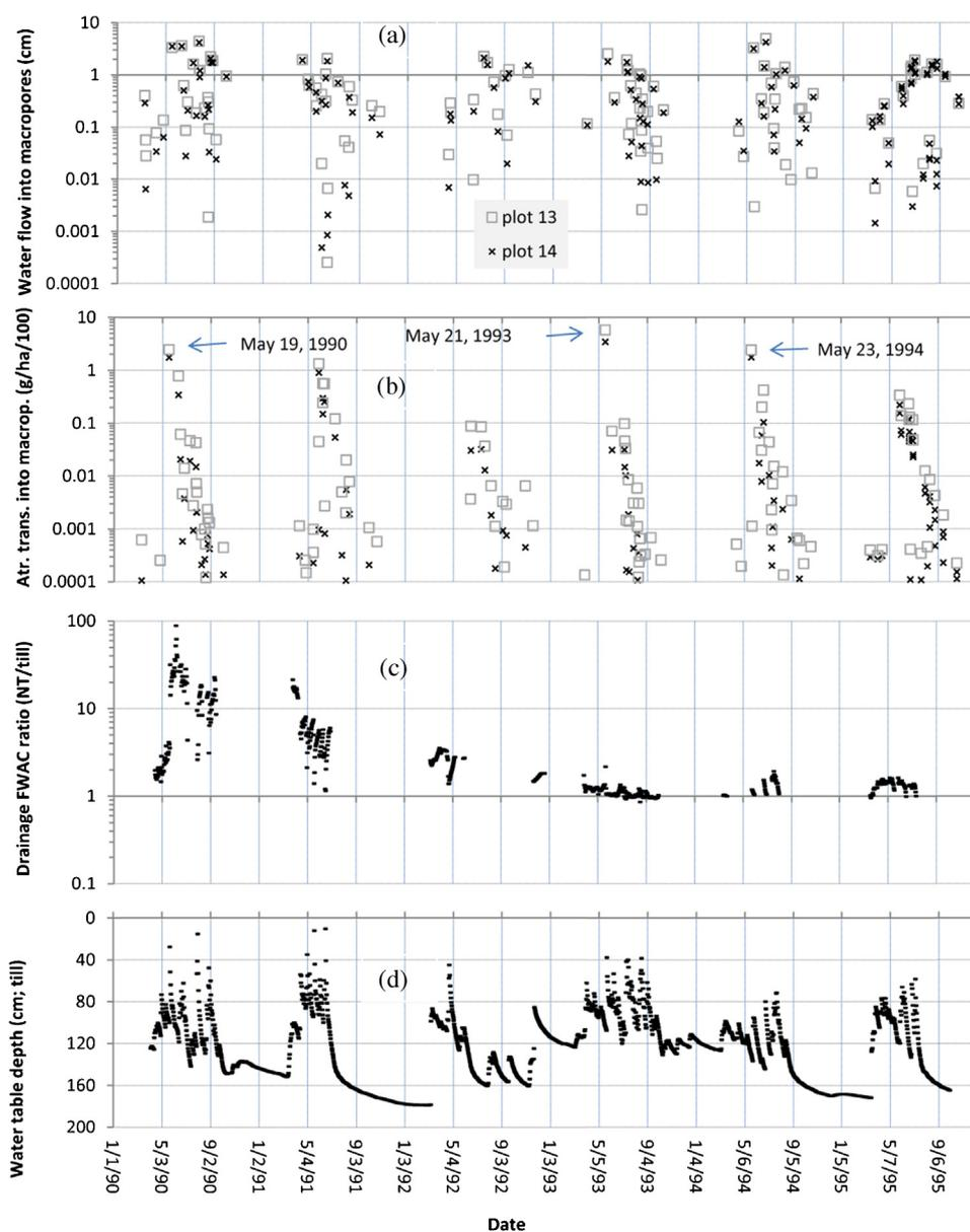
**Fig. 6.** RZWQM daily water table depth, atrazine concentration ratio in drain flow, and macropore flow characteristics. Atrazine was spring applied each year at a rate of 3 kg/ha for both plots 13 and 14. (a) is daily water flow into macropores. (b) is daily atrazine transport into macropores. (c) is daily flow weighted atrazine concentration (FWAC) ratio in drain flow (NT/till). (d) is daily water table depth for plot 13. Plot 13 is till and plot 14 is no-till (NT).
