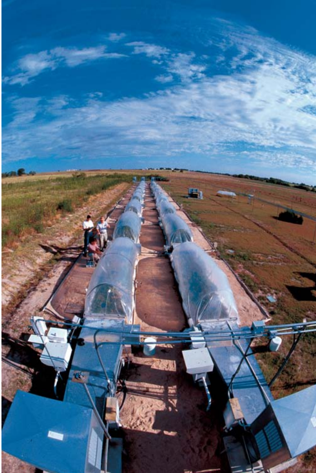
Figure 1. Field experiment at Temple, Texas, used to study the influence of increasing atmospheric CO 2 on mesic rangelands. Photo courtesy of Scott Bauer.
