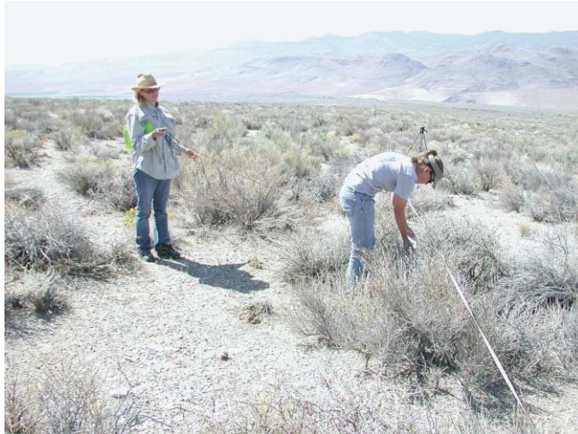
Figure 1. Mari-Vaughn Johnson and Julie Finzel taking vegetation measurements near Bishop, California. Plant physiological measurements can be taken with minimal disturbance using a ceptometer and clipping trials along vegetation transects in the field.
