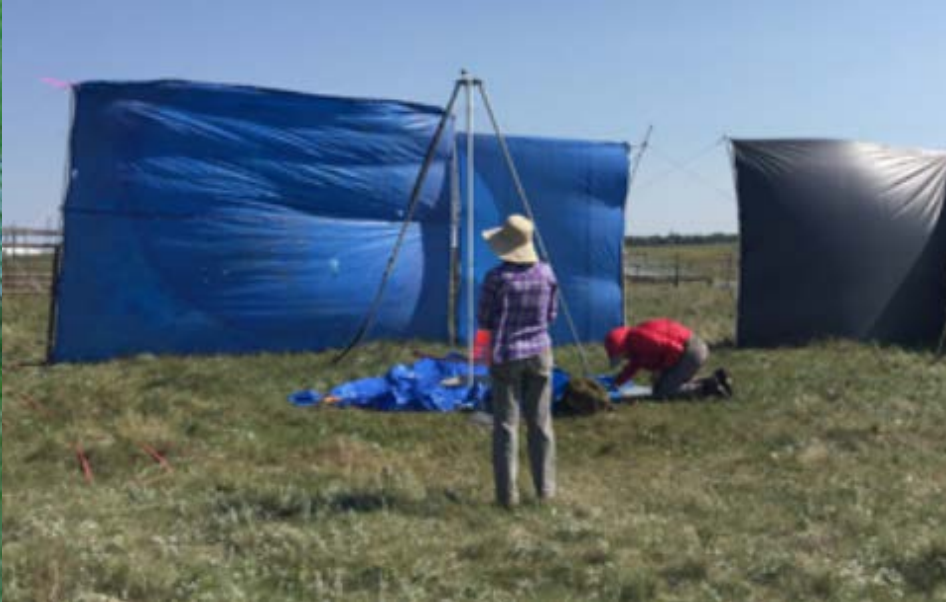
Two rainfall simulators being used to determine runoff in Kentucky bluegrass dominated rangelands.
