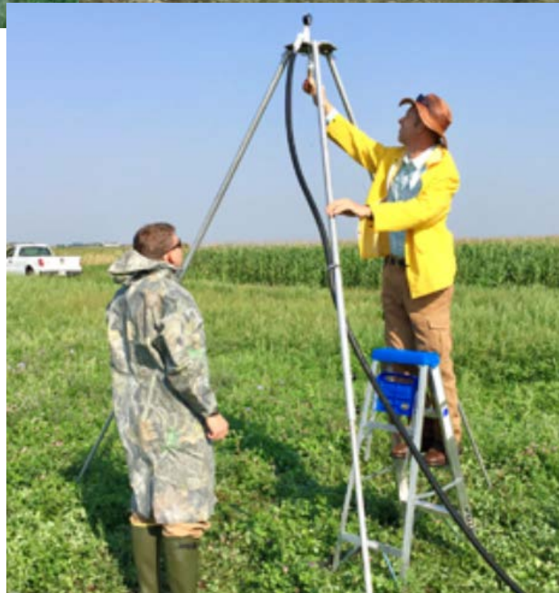
Setting up a rainfall simulator to determine runoff and runoff nutrient loads in an Integrated Crop Livestock Systems project.
