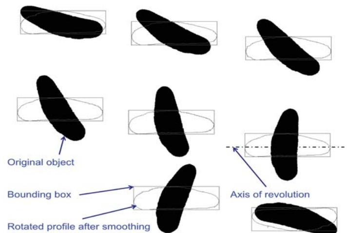
Fig. 3. Volume estimation of cucumber sample at several orientation showing original cucumber binary image, smoothed rotated profile representing about 240 discs, bounding box, and axis of revolution
