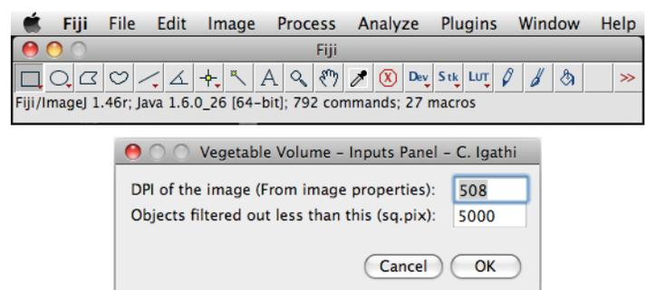
Fig. 2. Fiji/ImageJ image processing software and front panel of the developed volume estimation plugin program
