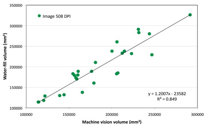
Fig. 4. Correlation and regression between machine vision and water-fill methods volume estimation
