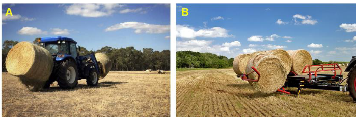
Figure 1. Examples of common and modern bale aggregation equipment: (A) Tractor equipped with bale spears at the front and rear (capacity = 1–2 bales); and (B) An automatic bale picker (ABP) with loading arm (capacity up to 23) - Image sources: https://www.himac.com.au and https://www.farm-king.com .
