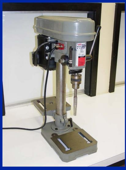
4. Coring devices must be in good condition and sharp or the core diameters will not be consistent and will result in spurious increased variation in shear values.
