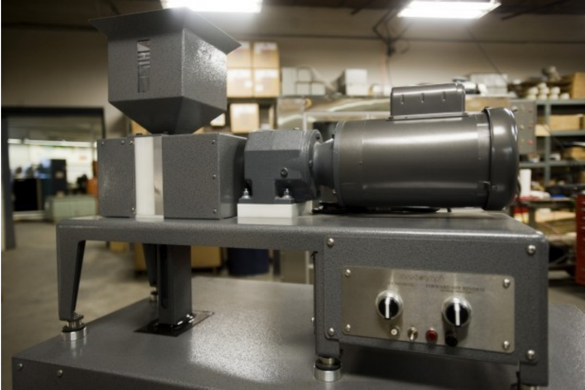
This machine developed by Dan Moore, Tom Pearson and Dan Brabec detects the presence of insect larvae in rice and wheat. (ERIN DUERR / Lincoln Journal Star)
