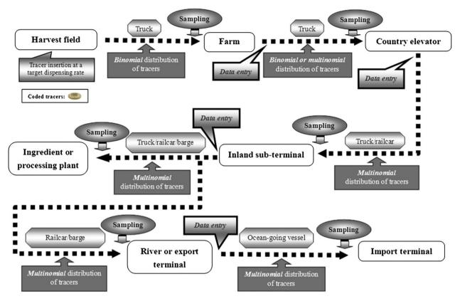
Fig. 1. General process flow diagram for the proposed grain tracing and recall system.
