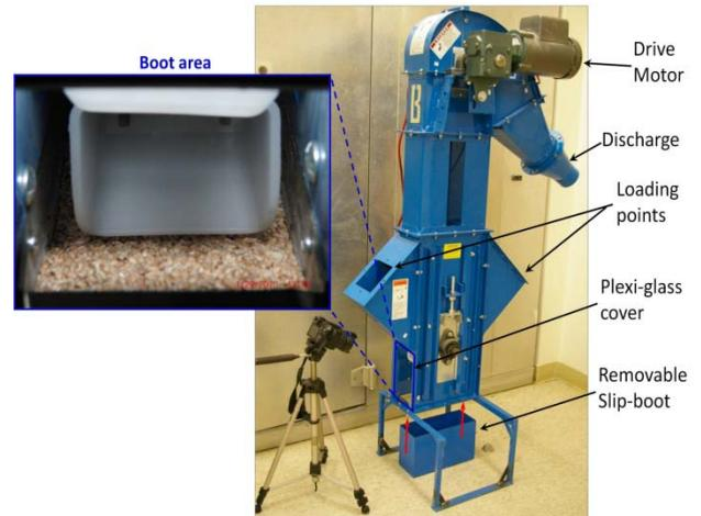
Figure 1. Pilot-scale bucket elevator leg boot arrangement.
