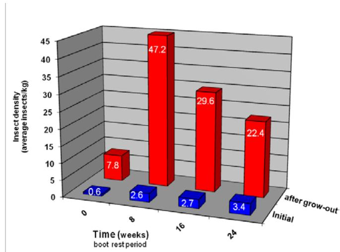
**Figure 3.** Average insect density in initially clean corn transferred over infested bucket elevator leg boots. Before the transfer, each infested boot was incubated for a 0, 8, 16, or 24 week rest period. After the transfer external insects were removed to obtain the initial count. After an 8-week grow-out period additional insects (emerged internal insects) were counted.
