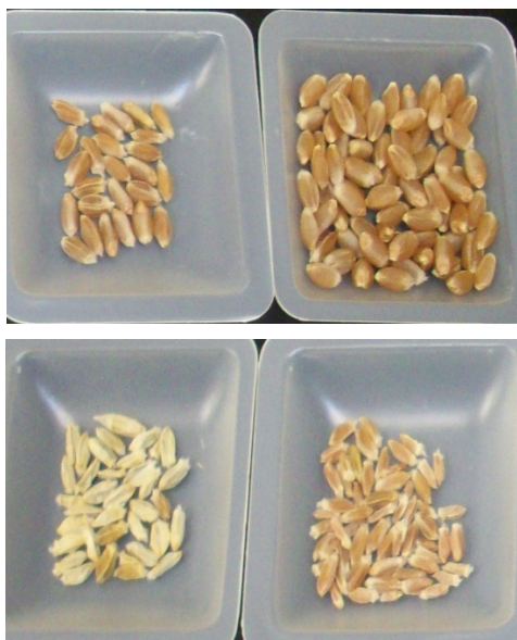
Wheat kernels undamaged (upper right) and with varying levels of fusarium damage, sorted by the SKNIR system.
