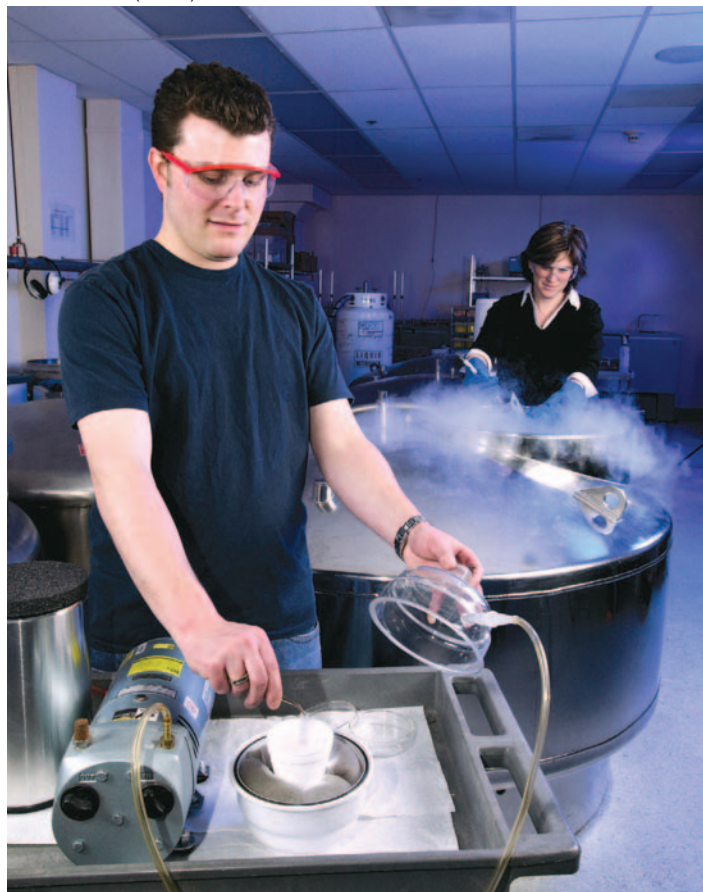
Technician Remi Bonnart (foreground) flash-freezes plant shoot tips while Christina Walters places cryopreserved materials into cryovats for long-term storage. Droplets of cryoprotecting solution hold shoot tips onto foil strips. The strips are plunged into liquid nitrogen slush that is formed by placing liquid nitrogen in a vacuum.
