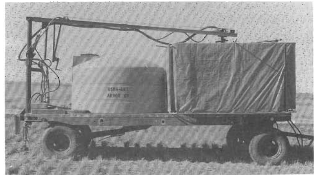
Figure 3—Rainfall simulator with the four-nozzle frame and enclosure in transport position.
