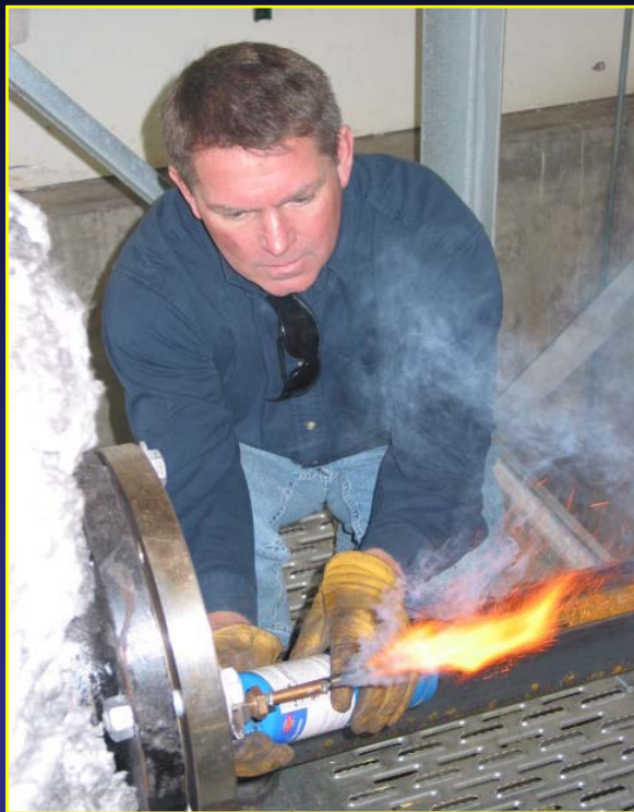
Ignited synthesis gas generated from straw
