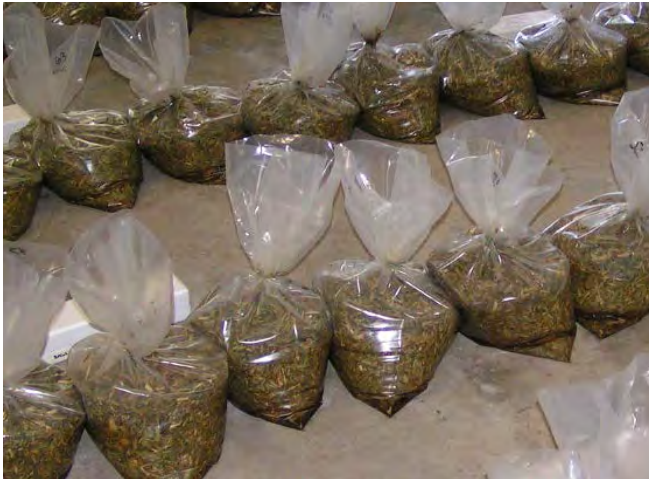
Figure 5. Soaking hay samples (each plastic bag contains 1 kg hay plus 5 L of 1% methyl- \beta -cyclodextrin in water). Courtesy of Leo den Hollander.
