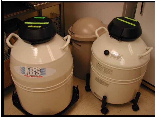
Storage Dewars for grass and hops cryopreservation
