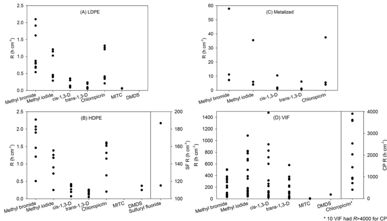
**Fig. 1.** Variation in the resistance to diffusion ( $R$ ) at  $25^\circ\text{C}$  of plastic films used in the Area-Wide Pest Management Project for each film type. All films were sampled directly from the roll with no field handling. HDPE, high-density polyethylene; LDPE, low-density polyethylene; VIF, virtually impermeable films.
