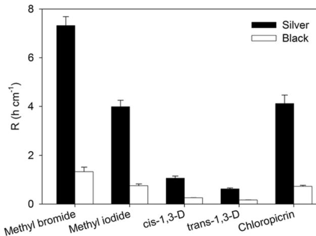
**Fig. 3.** Variation in resistance to diffusion ( $R$ ) factors for the transport of five fumigant compounds through different portions of a mixed composition film (silver indicates metalized and black low-density polyethylene). Values are the mean of three replicate cells; error bars indicate SE. All values determined for film with no field handling at 25°C.
