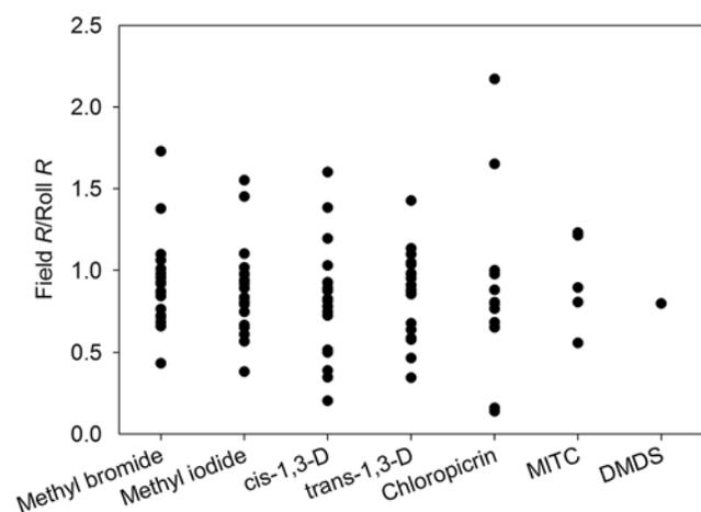
**Fig. 5. Ratio of the response of the resistance (*R*) value determined for VIF <48 h after field installation to that determined with no field handling (sample taken directly from the roll of film). All values determined at 25°C. Chloropicrin results do not include films for which both *R* values were not quantifiable in these tests (Supplementary Table S4). DMDS, dimethyl disulfide; MITC, methyl isothiocyanate.**
