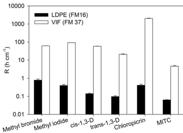
**Fig. 2.** Resistance to diffusion ( $R$ ) values determined at 25°C for six fumigant compounds through two films with no field handling. Values are the mean of triplicate cells; error bars indicate SE. Note that y axis is log scale. LDPE, low-density polyethylene; MITC, methyl isothiocyanate; VIF, virtually impermeable film.
