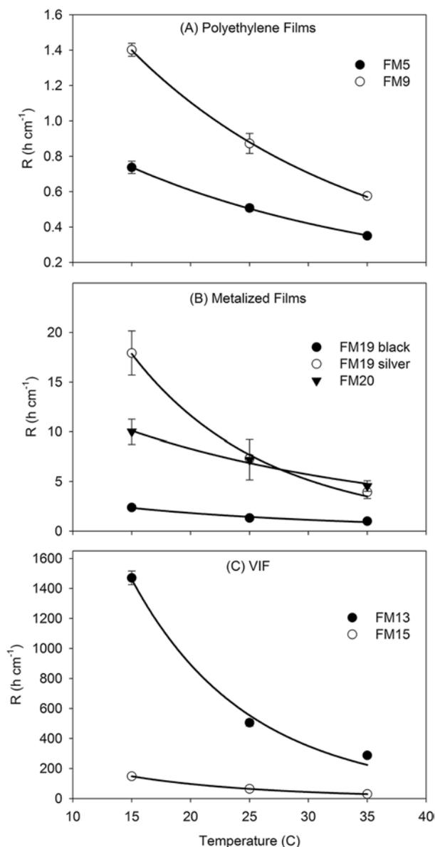
**Fig. 4.** Temperature response of the resistance ( $R$ ) of various films to methyl bromide diffusion. Values are the mean of triplicate measurements; error bars indicate SE. Lines indicate fit of the Arrhenius equation to the data. VIF, virtually impermeable films.
