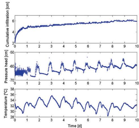
Fig. 4. Plots vs. time of (a) observed cumulative infiltration, (b) the applied pressure head at the rock surface, and (c) ambient temperature using an early high-tension infiltrometer prototype. Notice how the observed surface pressure heads are affected by the ambient temperature fluctuations.
