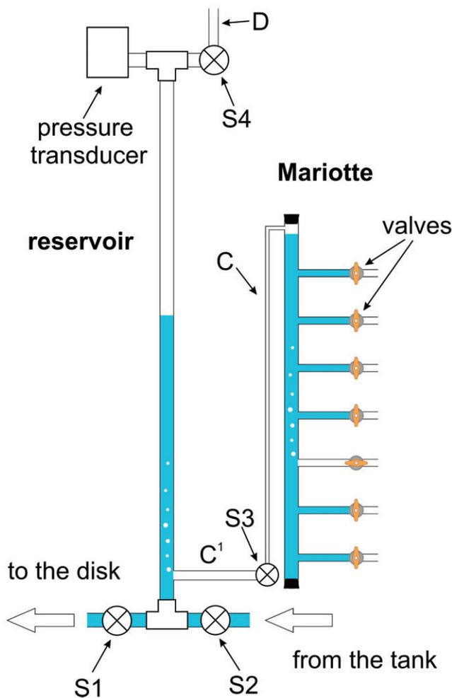
Fig. 3. Schematic of Mariotte and reservoir towers used for the improved low-flux, high-tension infiltrometer.
