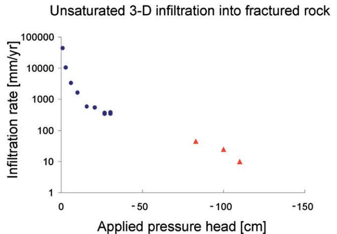
Fig. 6. Steady-state infiltration rates measured with a traditional soil tension infiltrometer (solid circles) and the improved low-flux, high-tension infiltrometer (solid triangles).
