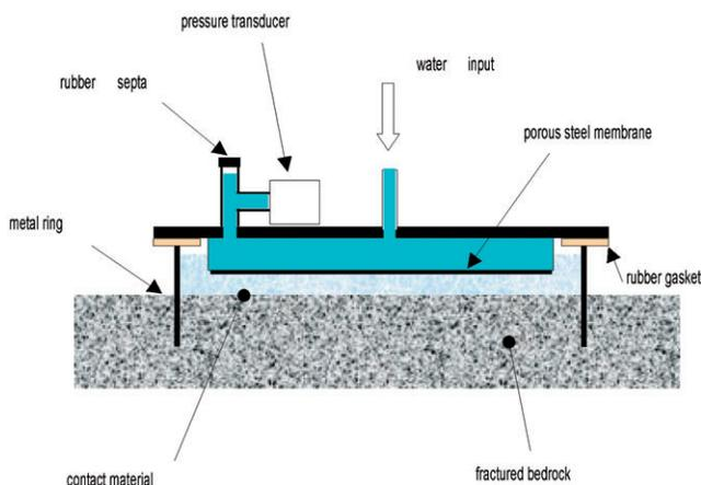
Fig. 2. Schematic of improved infiltrometer disk showing major components.
