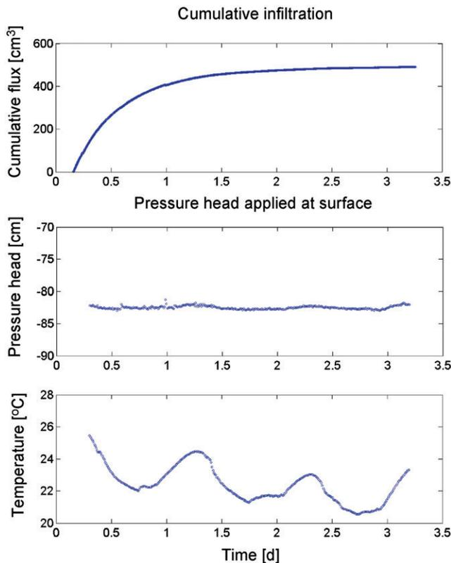
Fig. 5. Plots vs. time of (a) observed cumulative infiltration, (b) applied pressure head at rock surface, and (c) ambient temperature of the improved high-tension infiltrometer prototype. Notice that temperature fluctuations during this experiment were somewhat less severe as compared with the data in Fig. 4, system response was now much better. Surface pressure head variations were now  $<1$  cm, and without any noise in the cumulative infiltration data (Fig. 5a).
