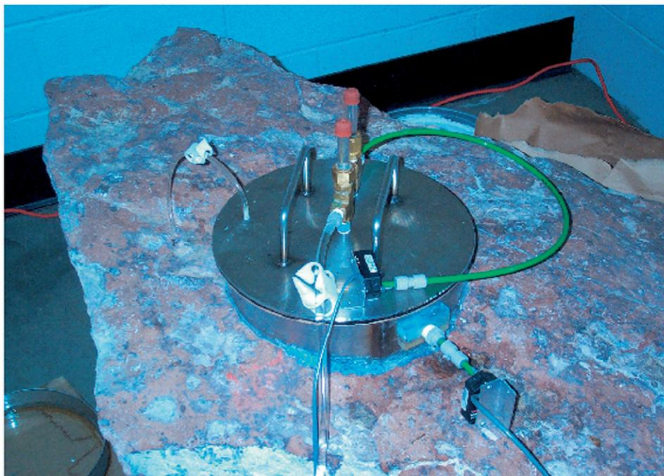
Fig. 1. View of improved tension infiltrometer disk setup on large fractured rock sample used in this study.
