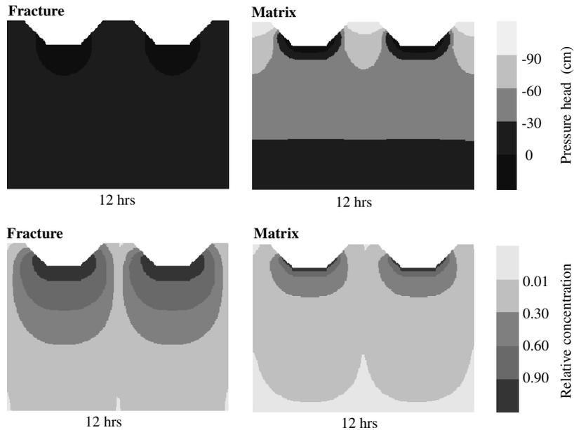
Fig. 5. Pressure head and concentration profiles in a dual-permeability system with uniform hydraulic properties (Scenario DU).
