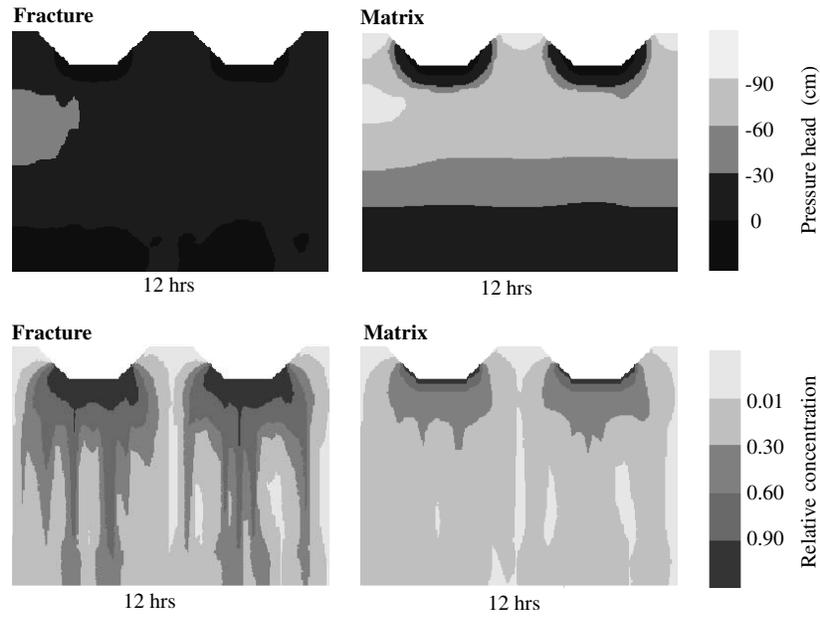
Fig. 6. Pressure head and concentration profiles in a dual-permeability system, in which the saturated hydraulic conductivity of the fracture domain was generated randomly (Scenario DRF).
