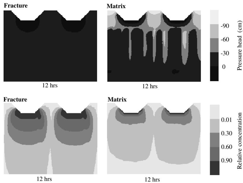
Fig. 7. Pressure head and concentration profiles in a dual-permeability system, in which the saturated hydraulic conductivity of the matrix domain was generated randomly (Scenario DRM).
