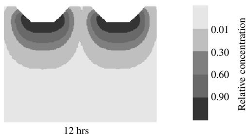
Fig. 2. Concentration profile at 12 h after the beginning of furrow irrigation in a single domain system with uniform hydraulic properties (Scenario SU).
