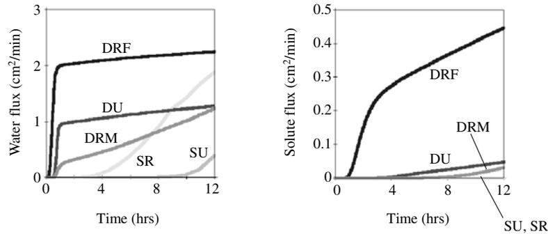
Fig. 8. Water and solute outflow from the lower boundary of the soil profile as computed for the respective flow scenarios: single uniform (SU), single with randomly generated conductivity (SR), dual uniform (DU), dual with randomly generated fracture conductivity (DRF), and dual with randomly generated matrix conductivity (DRM).
