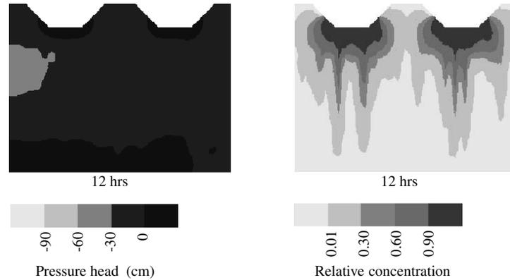
Fig. 4. Pressure head and concentration profiles in a single domain system with the randomly generated conductivity field (Scenario SR).
