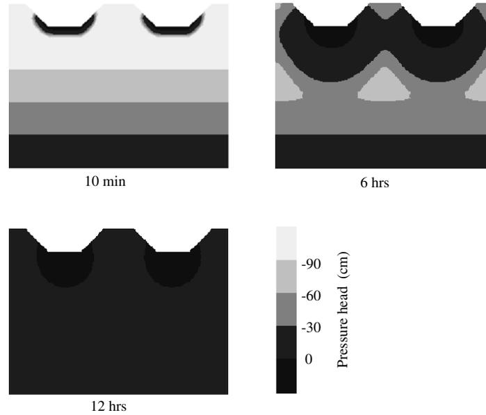
Fig. 1. Pressure head profiles at 10 min, 6 and 12 h after the beginning of furrow irrigation in a single domain system with uniform hydraulic properties (Scenario SU). The size of the flow domain is  $2.0 \times 1.5 \text{ m}^2$ .
