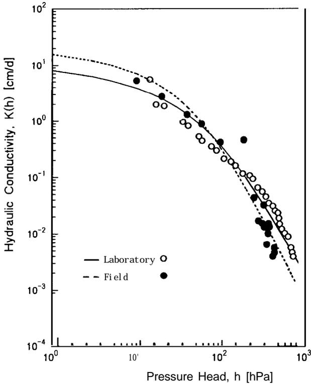
Fig. 7. Measured and fitted curves for the field and laboratory conductivity (Case 1;  $\theta_t = 0$ ).
