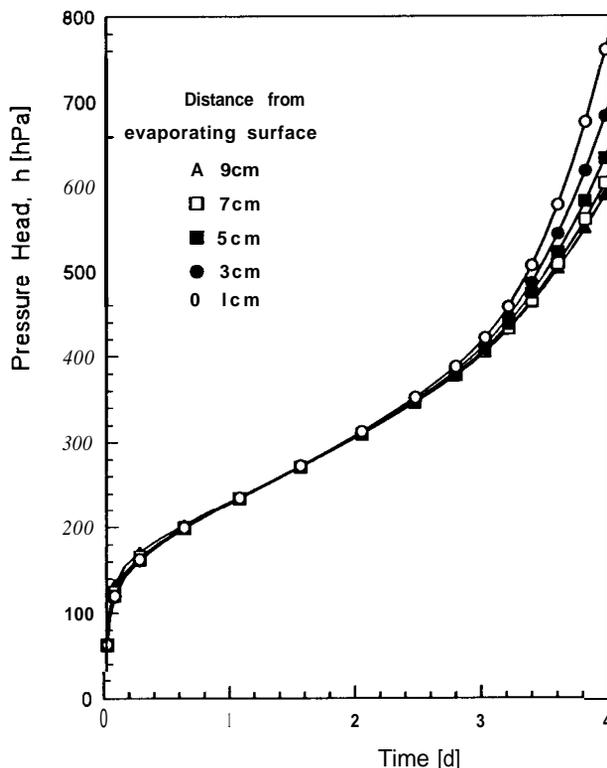
Fig. 4. Soil water pressure head, measured with tensiometers at five positions in the soil column, as a function of
