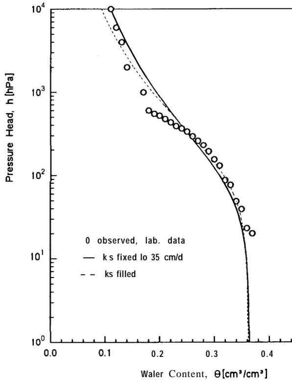
Fig. 10. Measured and fitted curves with  $k$ , fitted or fixed to the value measured with the constant-head permeameter for the laboratory retention (Case 4).
