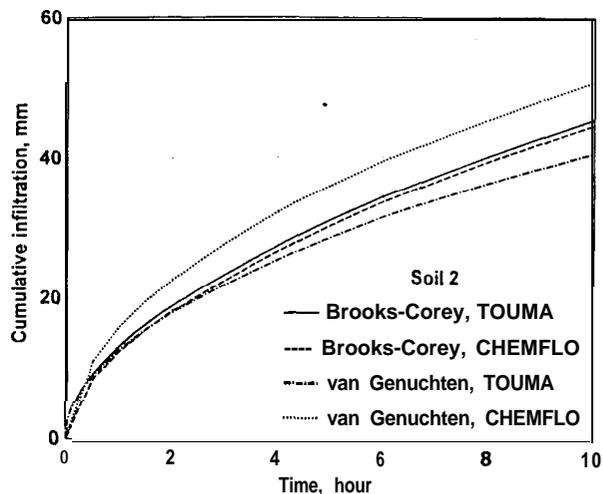
Figure 5. Cumulative infiltration depth as a function of time for soil number 2 in Table 1, using the BC or vG expressions according to the proposed equivalence and as calculated with the two numerical codes, CHEMFLO and Touma's [1984].
