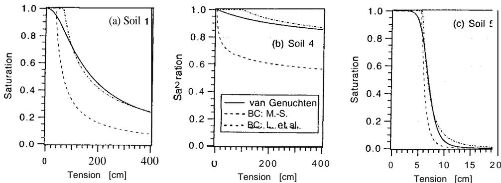
Figure 8. Saturation as a function of tension (centimeters) for soil numbers (a) 1, (b) 4, and (c) 5 used in Lenhard et al.'s [1989] paper, using the vG expressions and the BC expressions according to the proposed M-S equivalence and the Lenhard et al. equivalence.
