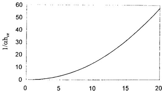
Figure 1. Dimensionless ratio  $(1/\alpha)/h_{ce}$  as a function of the parameter  $p$ , exponent of normalized water content for the power law expression of relative permeability.
