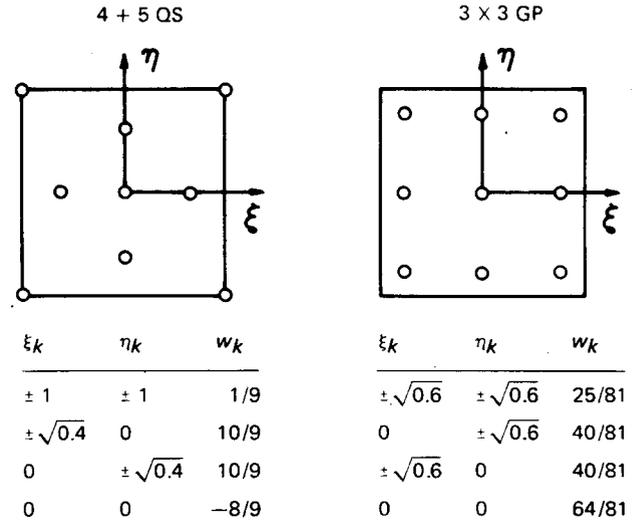
Figure 2. Location of integration points and values of weighting coefficients for the nine-point Lobatto-type (4 + 5 QS) and nine-point Gaussian quadrature (3 x 3 GP) schemes
