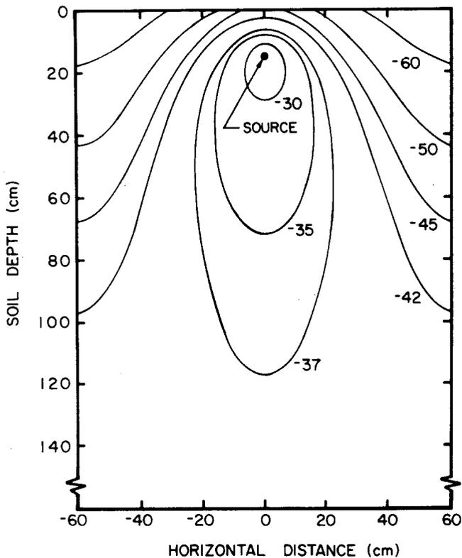
Figure 6. Calculated steady-state pressure head distribution resulting from a buried line source at  $z = -15$  cm (semi-infinite profile)
