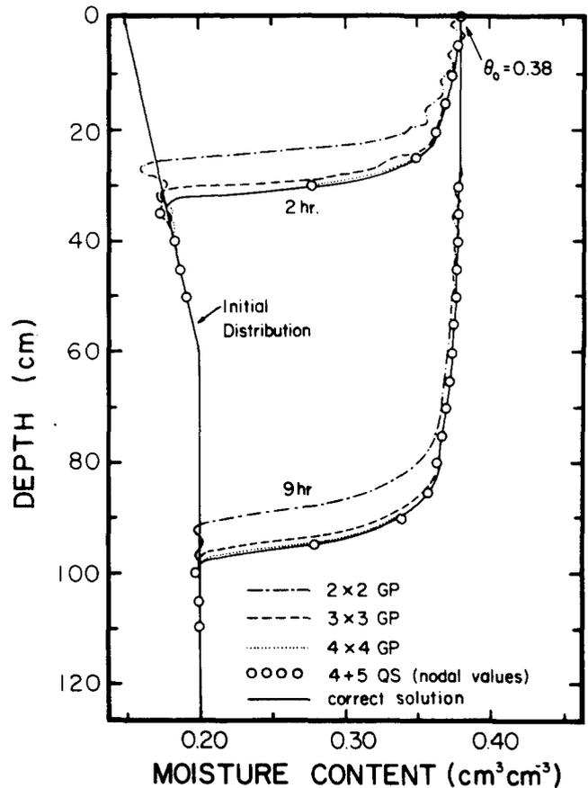
Figure 3. Effect of different quadrature schemes on computed moisture distributions
