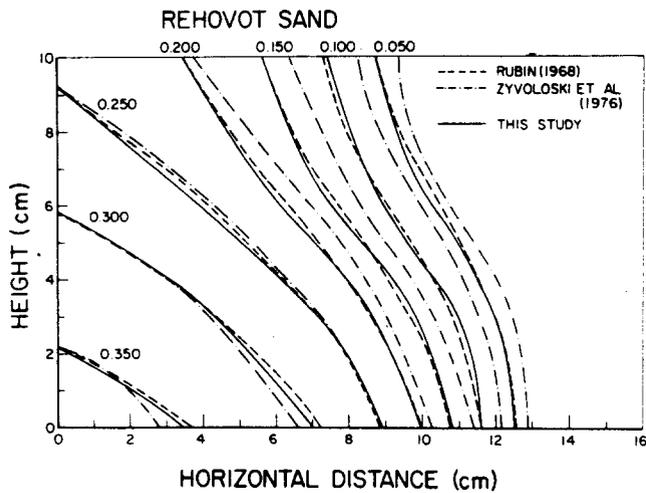
Figure 4. Calculated moisture distributions during infiltration into a horizontal soil slab
