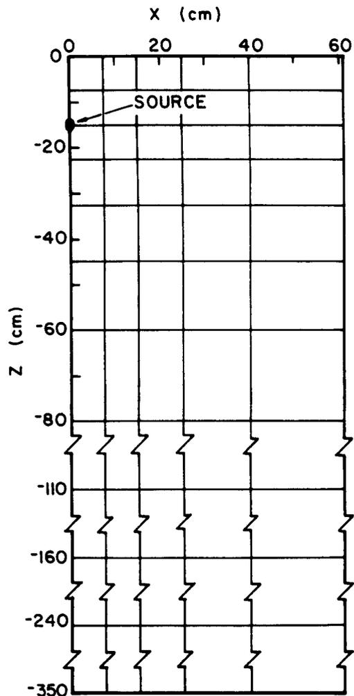
Figure 5. Schematic representation of the line source problem and the associated finite element mesh
