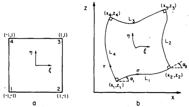
Figure 1. Deformed isoparametric Hermitian elements in local (a) and global (b) coordinates
