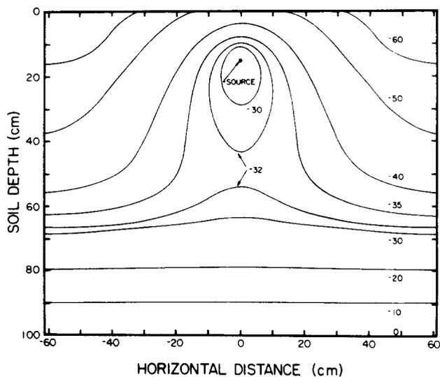
Figure 7. Calculated steady-state pressure head distribution resulting from a line source at  $z = -15$  cm (fixed water table at  $-100$  cm)
