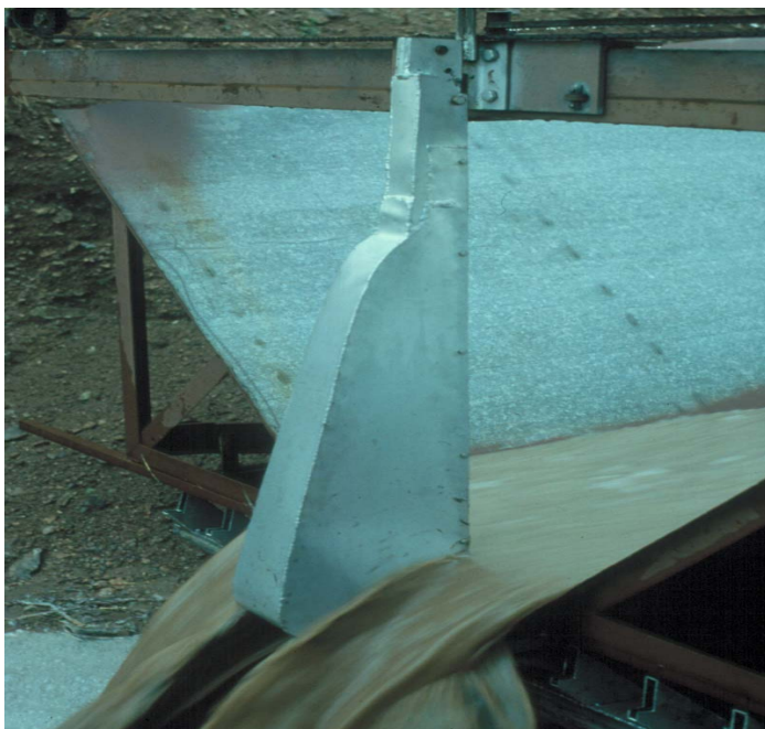
Traversing slot sediment sampler collects sediment samples during a flow event.
