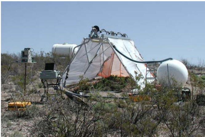
The Walnut Gulch Rainfall Simulator setup for a field experiment.
