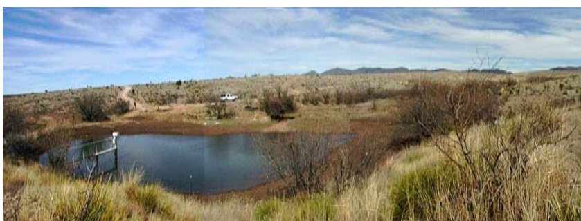
Sediment yield is monitored at stock ponds located at the outlets of 10 small watersheds.
