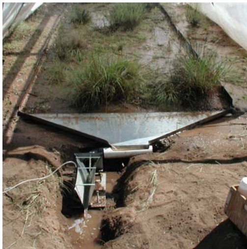
Plot scale rainfall simulator sediment yield experiment.
