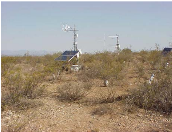
Eddy covariance, Bowen ratio and sap flow sensors at Lucky Hills.
