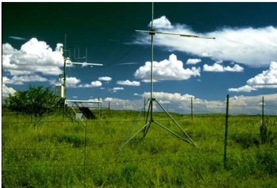
Bowen ratio system at the Walnut Gulch Experimental Watershed grassland study site used to measure carbon dioxide and water vapor movement.
