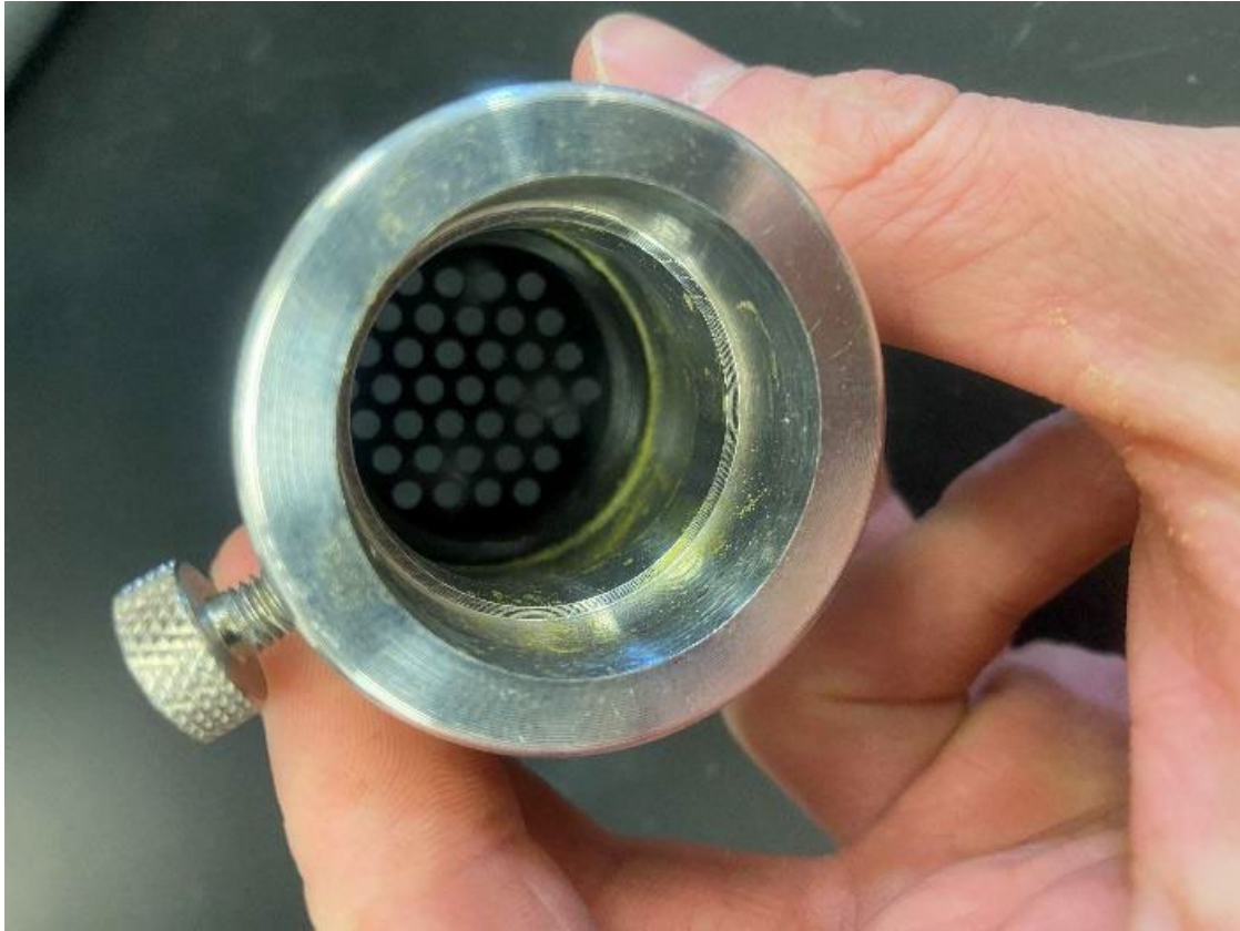
Figure 3: Pollen can collect along internal grooves and corners of the collection apparatus.
