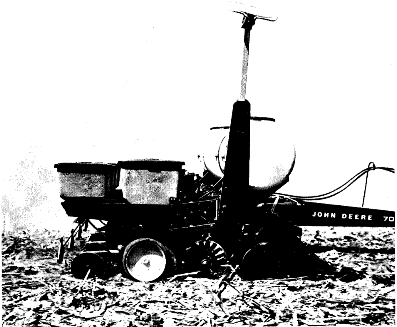
Figure 8. Fluted coulters, located in the front of the no-till planter, open a 2 inch slot for seed placement. Otherwise, the soil is not disturbed.
