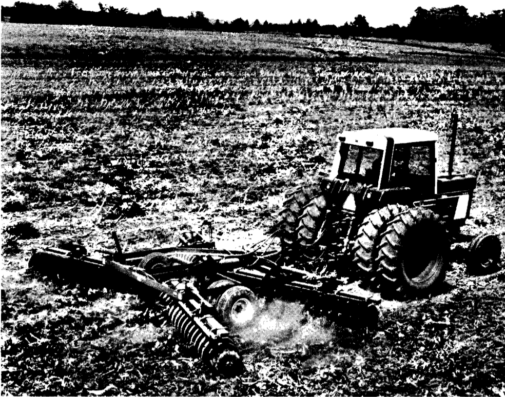
Figure 3. Large-bladed offset or tandem disks are now used by many farmers for primary tillage.
