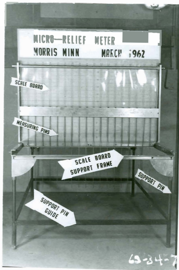
Figure 2.--Micro-relief meter showing support pins and support pin guide.
