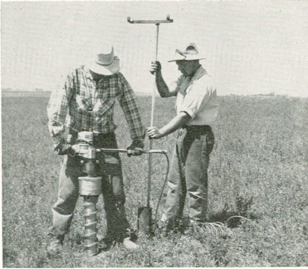
Figure 3—Soil sampler used to obtain undisturbed soil cores. The core was sectioned into 3-inch increments for bulk density determinations.
