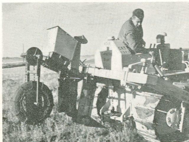
Figure 2—Subsoiler with fertilizer applicator. The ground wheel drove the fertilizer metering device, and the rear shank led the fertilizer to the bottom of the subsoiled channel.
