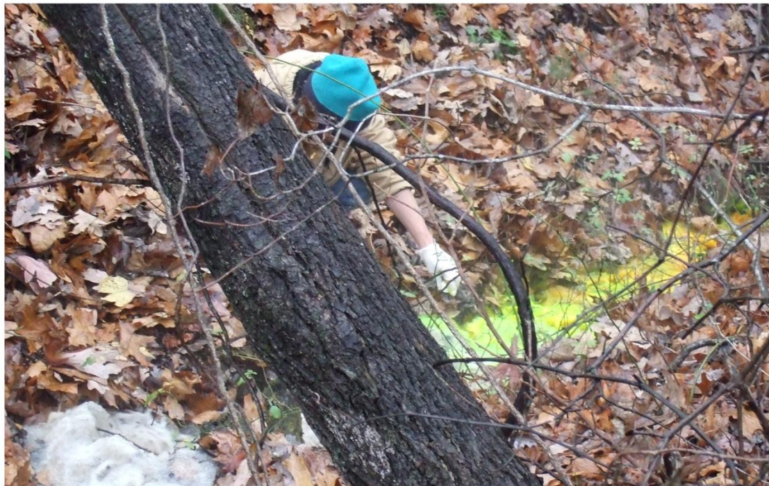
Figure 12: Injecting fluorescein near Nixon School Road, 11/26/2007.
