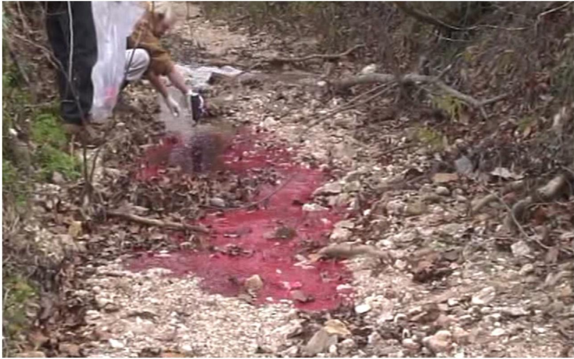
Figure 6: Injecting rhodamine WT into Avery Hollow at Land Town Loop Road, 11/1/2006.
