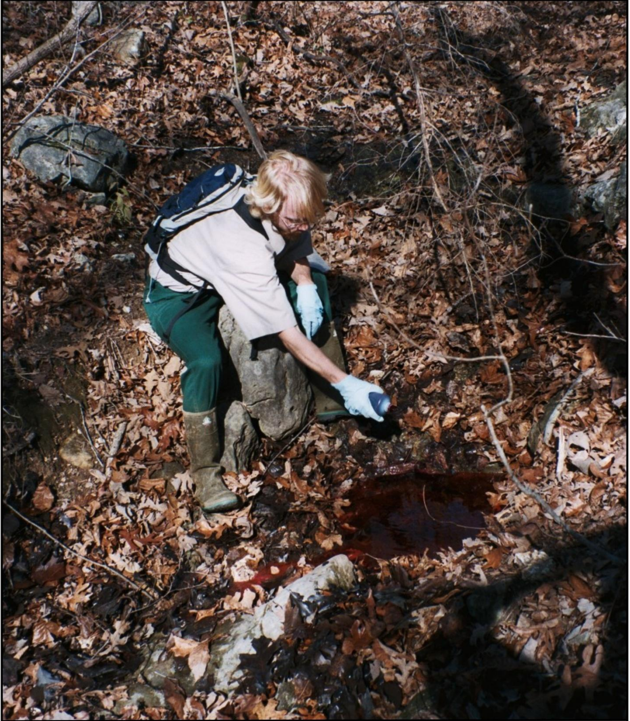
FIGURE 4: BEN MILLER INJECTING RHODAMINE WT INTO “DEAD FROG” HOLLOW, 11/11/2003.
