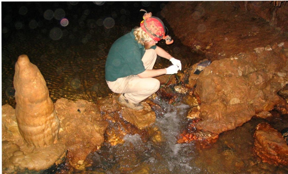
Figure 10: Ben Miller changes a charcoal receptor in Lost River, within Onondaga Cave.
