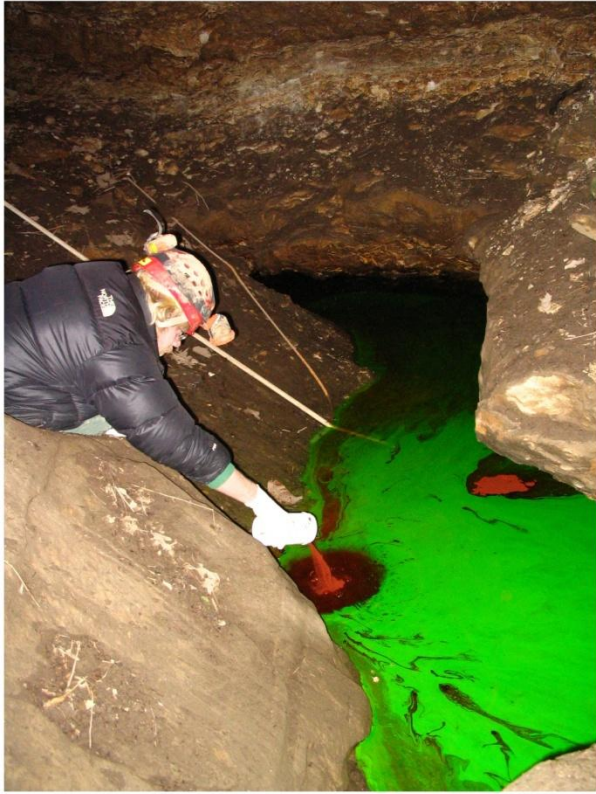
Figure 8: Ben Miller injects fluorescein into Snake Pit, 1/18/2005.
