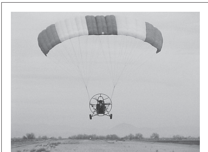
Figure 6. A powered parachute as a sensor platform in Tucson, Arizona.
