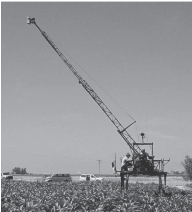
Figure 4. A boom-type data acquisition system mounted on a high-clearance tractor at the ARS Water Management Research Center in Ft. Collins, Colorado.
