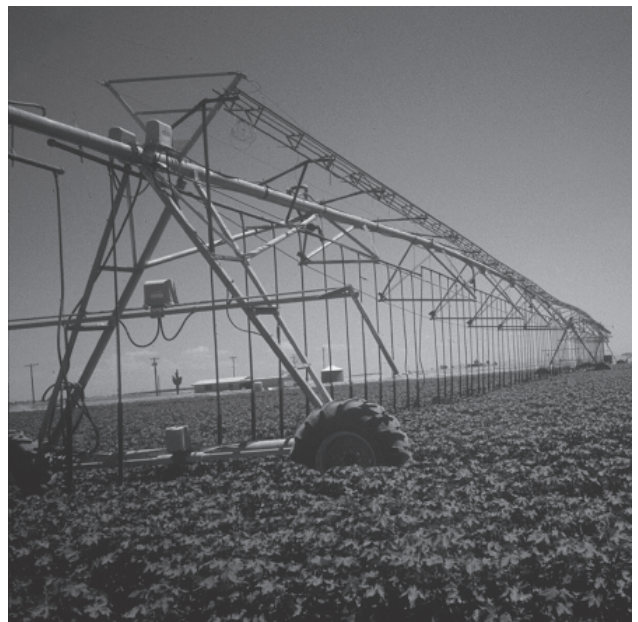
Figure 5. The linear move system serving as a platform for the Agricultural Irrigation Imaging System, AgIIS Ag Eyes, in Phoenix, Arizona.
