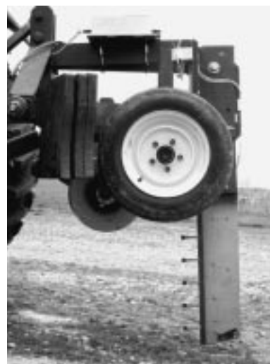
Side view of the SSPS raised out of the ground, showing the five sensing tips.
