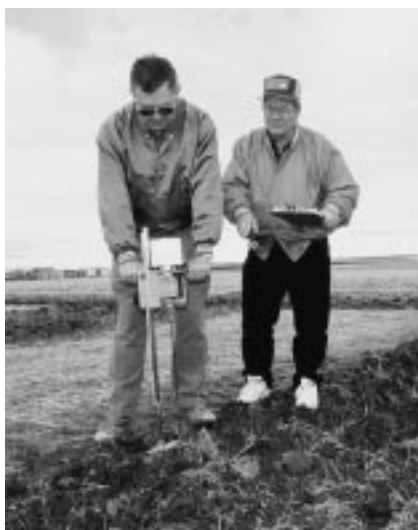
Researchers collect soil strength measurements with a recording cone penetrometer. (Photo by Scott Bauer, courtesy of USDA-ARS)
